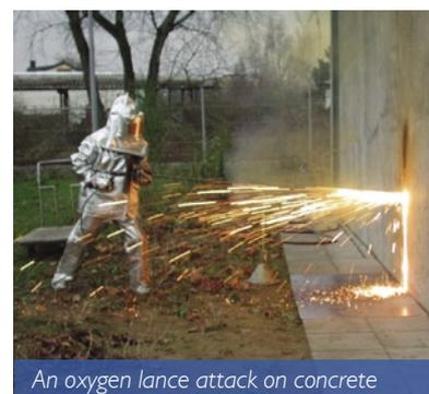
*An oxygen lance attack on concrete*
